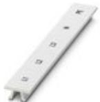
Zack marker strip, Strip, white, labeled, printed horizontally: L1, L2, L3, N, PE, mounting type: snap into tall marker groove, for terminal block width: 15.2 mm, lettering field size: 10.5 x 15.1 mm, Number of individual labels: 5
