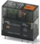
Plug-in miniature relay, with multi-layer contact with hard gold coating, 1 changeover contact, test button, mechanical switching position indicator, status LED, input voltage 230 V AC
