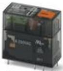
Plug-in miniature relay, with power contact, 2 changeover contacts, test button, mechanical switching position indicator, status LED, coil voltage 230 V AC
