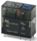
Plug-in miniature relay, with multi-layer contact with hard gold coating, 1 changeover contact, test button, mechanical switching position indicator, status LED, freewheeling diode, polarity A1+, A2-, input voltage 24 V DC
