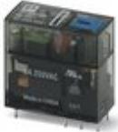
Plug-in miniature relay, with multi-layer contact with hard gold coating, 2 changeover contacts, test button, mechanical switching position indicator, status LED, freewheeling diode, polarity A1+, A2-, input voltage 24 V DC
