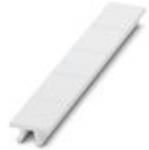
Zack marker strip, Strip, white, unlabeled, can be labeled with: PLOTMARK, CMS-P1-PLOTTER, mounting type: snap into tall marker groove, for terminal block width: 15.2 mm, lettering field size: 10.5 x 15.1 mm, Number of individual labels: 5
