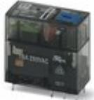
Plug-in miniature relay, with power contact, 1 changeover contact, test button, mechanical switching position indicator, status LED, freewheeling diode, polarity A1+, A2-, input voltage 24 V DC
