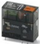
Plug-in miniature relay, with power contact, 2 changeover contacts, test button, mechanical switching position indicator, status LED, coil voltage 120 V AC
