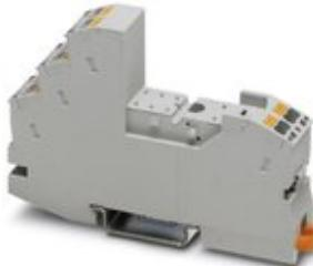
Relay base RIF-1..., for miniature power relay with 1 or 2 changeover contacts or solid-state relays of the same design, Push-in connection, plug-in option for input/interference suppression modules, for mounting on NS 35/7,5
